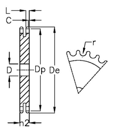
C = 1 D = 14 De = 110.4 Dp = 106.26 For chain size =  $3/8 \times 7/32$ For chain type = 06 B-2
